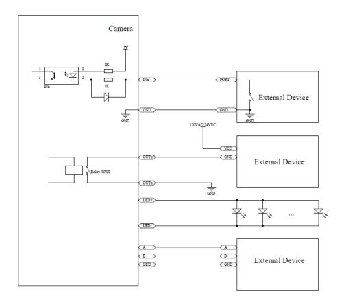
**Chart 2-2 Common Interface Wiring Diagram**
